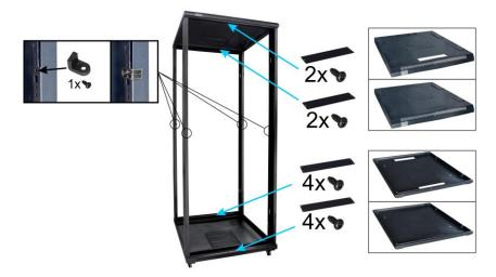
5.4) Inside the cabinet, install the cross profiles, distance and RACK profiles from the inside (front and rear), as shown in the figure below.
